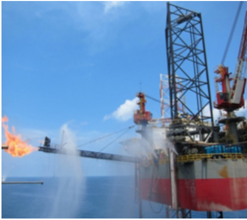
CO 2 injection and flow back operation using the rig and the supply boat
